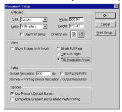
Put check in [Use Print Setup] and click the [Print Setup] button.
